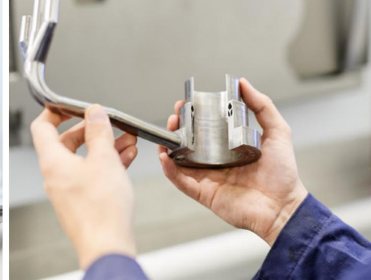
Fuel nozzle with internal heating ducts
